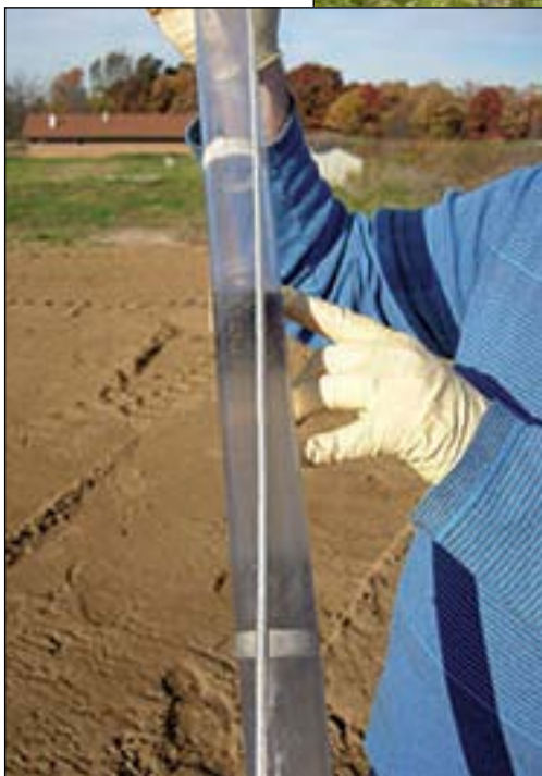
Measuring the amount of scum in a septic tank
